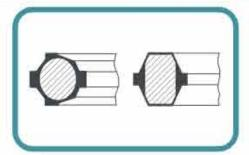
This (oval or octagonal) type is widely used during test procedures. Another advantage is that with the proper use of this gasket, it can be re-used.
