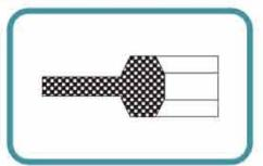
Blind ring type joints can be manufactured to blank off flanges and pipe work. They consist of standard Ring Type Joints with integral solid metallic centers.
