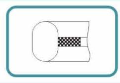
PTFE Loose Inner Ring. The purpose of this ring is to prevent corrosion of the gasket and flange grooves by the contained medium.
