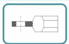
A Ring Type Joint Gasket fitted with a sponge rubber outer ring to prevent corrosion from atmosphere.
