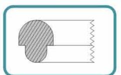
Transition Ring Type Joints are used when the flanges have different groove dimensions or profiles. Transition Ring Type Joints are available with either oval or octagonal facings and are not encompassed by the API specification.
